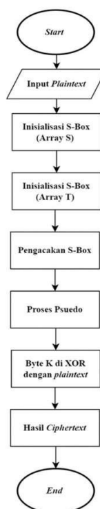
Flowchart Enkripsi RC4
