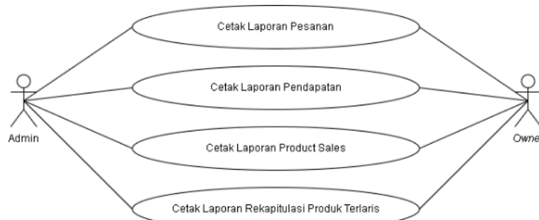
Gambar 7. Use Case Diagram Laporan
