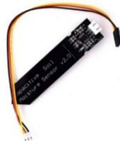
Gambar 1. Sensor Kelembaban Tanah
