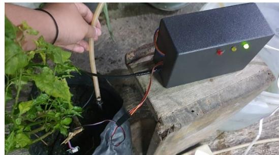
Gambar 10. Membaca Sensor Kelembaban Tanah
