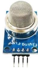
**Gambar 8.** Sensor asap ( Sensor MQ2)
