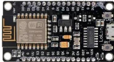
Gambar 5. NodeMcu ESP8266
