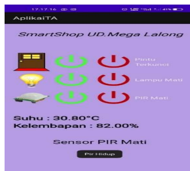
Gambar 11. Tampilan monitoring sensor pir
