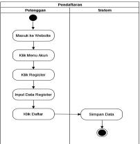
Gambar 4. Activity Diagram Sistem Usulan Pendaftran
